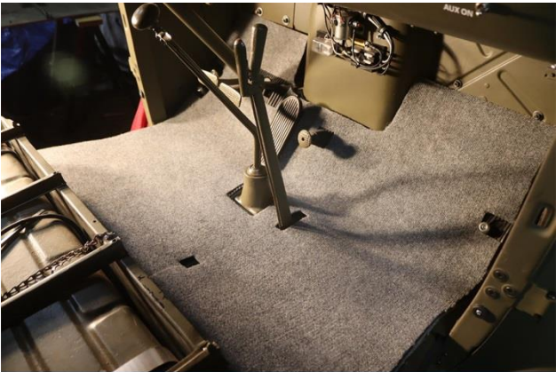
Thin carpet material fit over the cab floor to protect the rubber floor mat.
