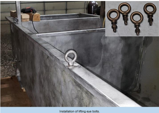
Installation of lifting eye bolts.
