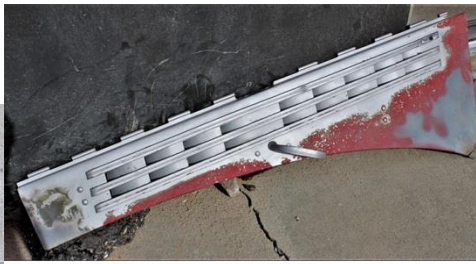
The complexly vented hood side-panels were bead-blasted to remove many layers of paint. The damaged uppermost spear on this panel will be replaced.
