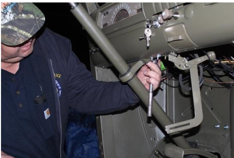
John Gudgeon tightens bolts on the steering column support bracket.
