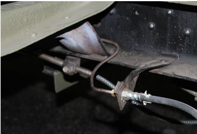
Mike Johnson fabricated a new chassis brake line and installed it.
