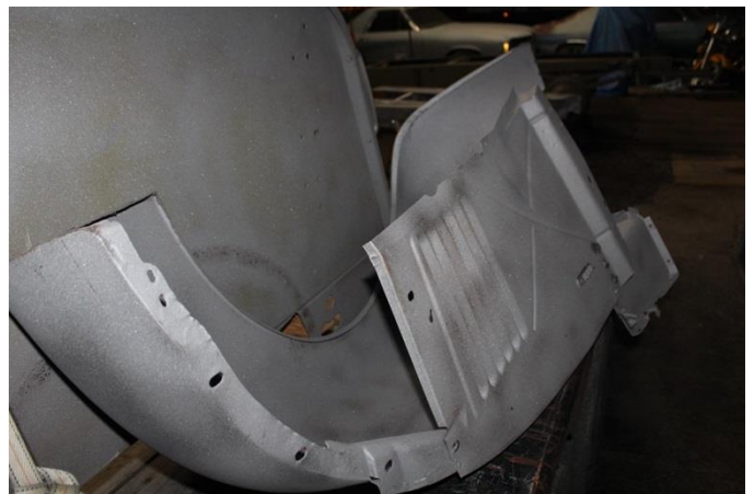
Jerry Russell and Doug Walters are figuring the best way to detach, paint, and reattach the fender inner panels.
