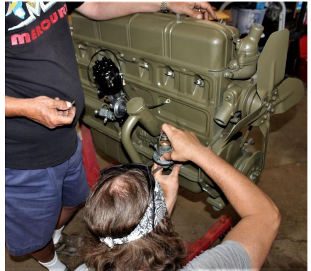
Ty and Jerry install the restored fuel pump. Note restored distributor.
