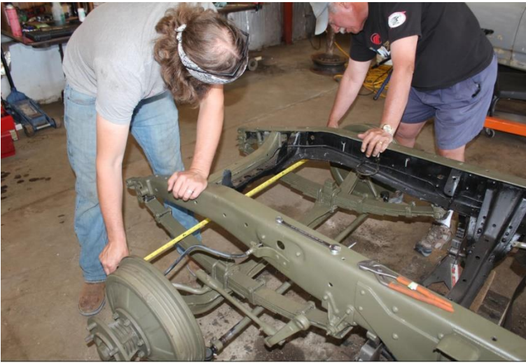
Ty Clinton and Jerry Russell set toe-in after installing the tie rod.
