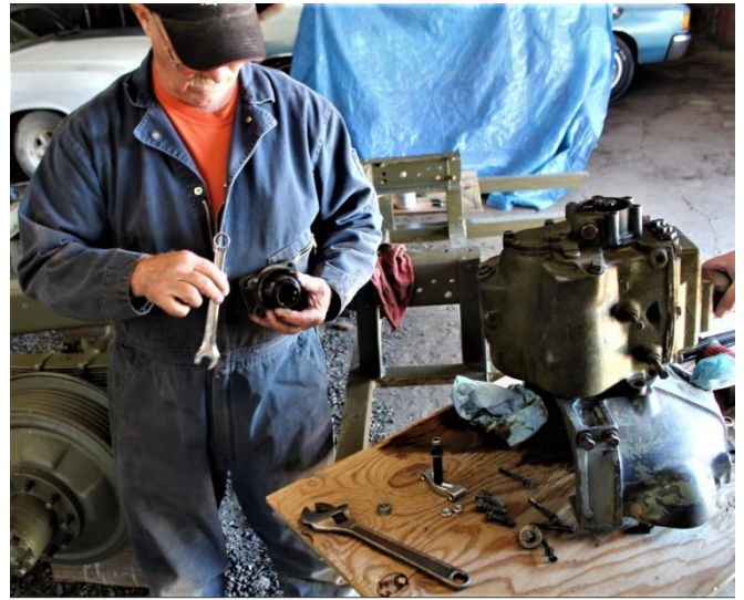
Mike Johnson inspects the transmission output seal.
