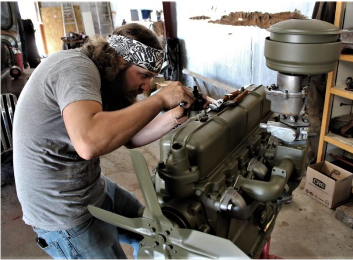
Ty installs the new ignition coil. Note the governor, carburetor, and air cleaner.
