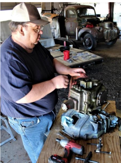
John Gudgeon cleans the transmission and bellhousing.
