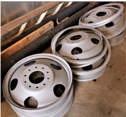
The wheels are sandblasted and ready for paint. Once the wheels are painted, tires will be ordered.
