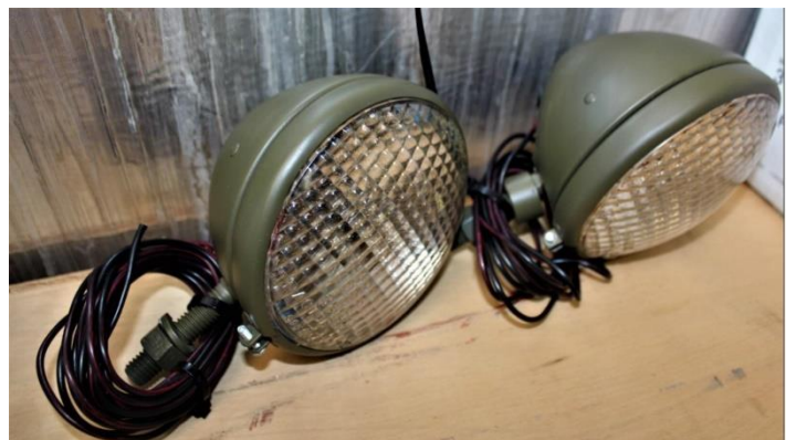
The rear flood lights have been restored and are ready for installation
