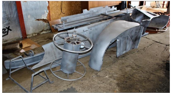
Other prepped items include fenders, bumper, skirting, and fire equipment.
