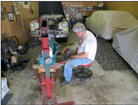
Mike and Mark mating transmission to engine
