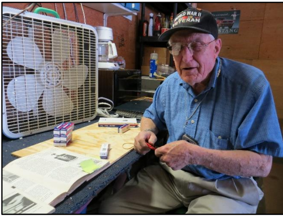
Wally gaps a new set of spark plugs for the engine
