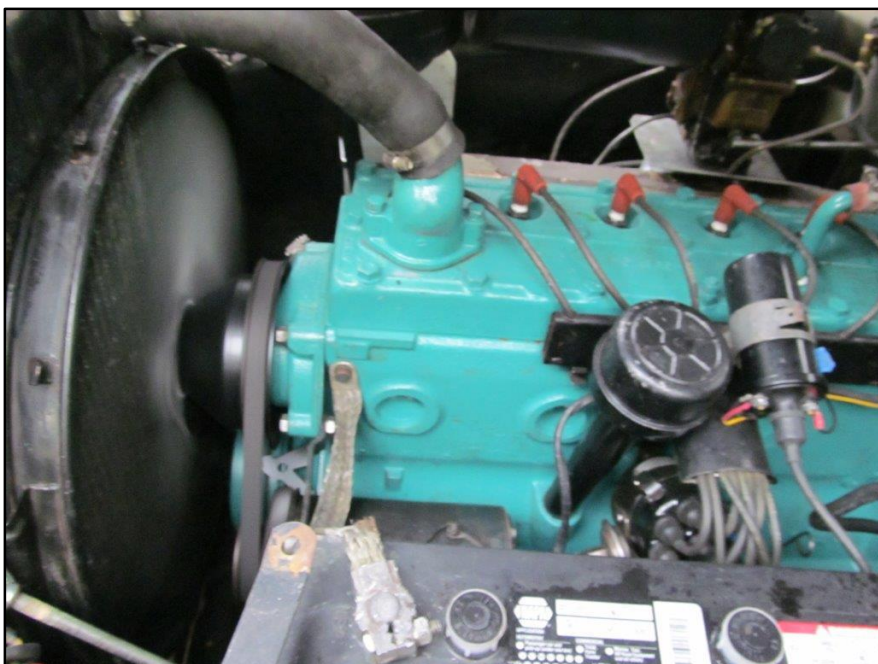
Eight happy cylinders of straight eight Pontiac power ready for new adventures
